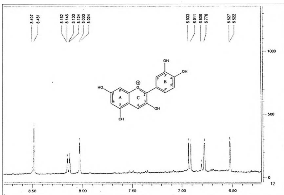
Figure 4.4 ^1\text{H-NMR} spectrum of cyanidin extracted from red cabbage
