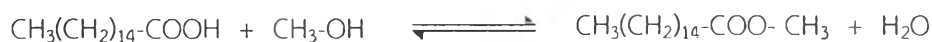
Figure 1.3 Esterification of free fatty acid and methanol to produce fatty acid methyl ester and water as products [11].
