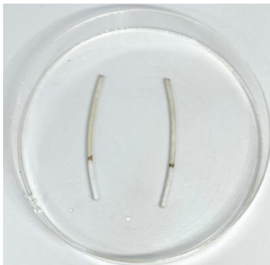
Figure 4.27 PLA that soaked into 50 and 100 mM AgNO 3 .
