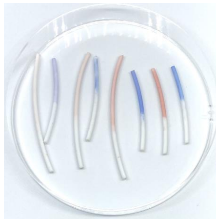
Figure 4.11 3,4,5,6,7,8,9,10 layers of PEMs deposited filament appearance respectively.
