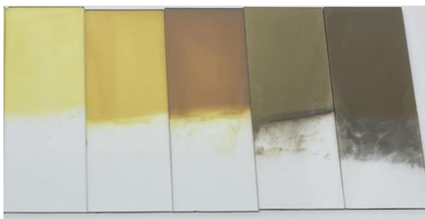
Figure 4.5 Silver nanoparticles coating on PEMs at different concentration of PSS-co-MA 0.25, 0.1, 0.05, 0.01, 0.005 mM respectively.
