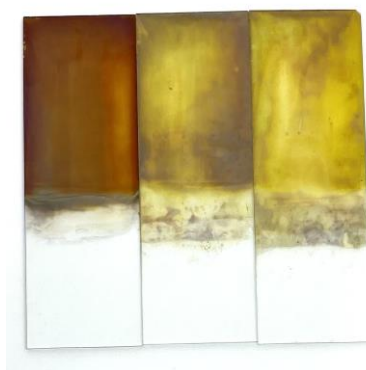
Figure 4.10 DI water, PSS 50 mM → NaCl 2 M, NaCl 2 M → PSS 50 mM respectively.
