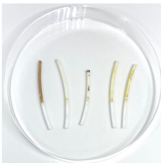
Figure 4.28 PLA with 8,10,12,14,16 PEMs layers using 10 mM AgNO 3 respectively.
