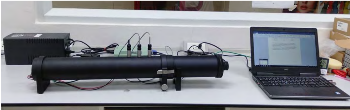
Figure 2.5 Impedance tube kit with large tube
