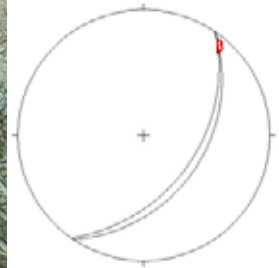
Figure 4.3 Kink folds at Khao Wua illustrating axial plane dipping to SE. Fold axis is 40/7 (trend/plunge). Grid reference 0713055 E 1409002 N.
