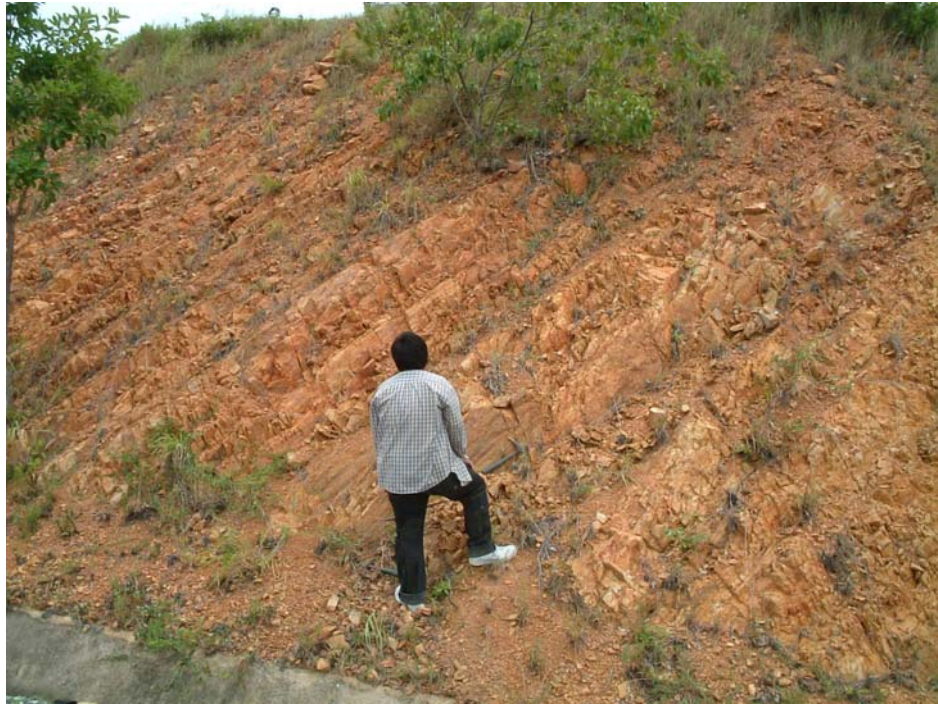
Figure 3.27 Bedding of quartzite at Khao Laem Chabang (Sri Racha III). The attitude of bedding is (strike/dip) 212/40 NW. Grid reference 0703520 E 1446150 N.
