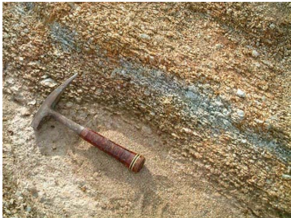
Figure 3.42 Highly weathered foliated granite at the same locality as in Figure 3.4.
