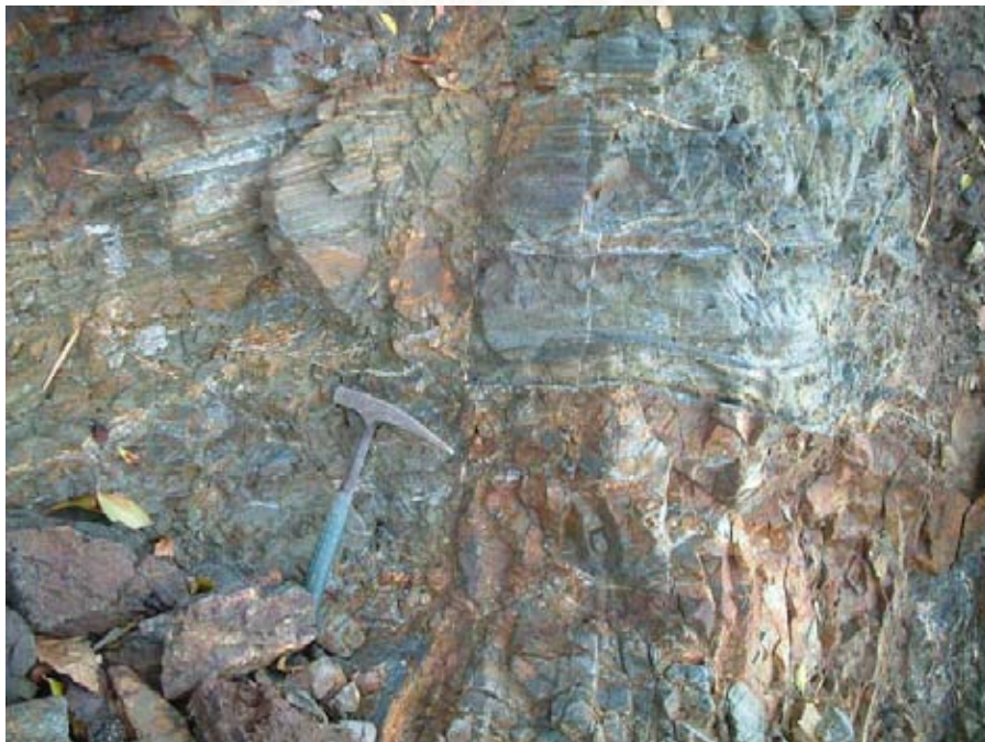
Figure 3.7 Shale intercalated with grayish black sandstone with joints and irregular fractures directions (Sattahip I). Bedding attitude is 348/31 NE. Grid reference 0701951 E 1411488 N.
