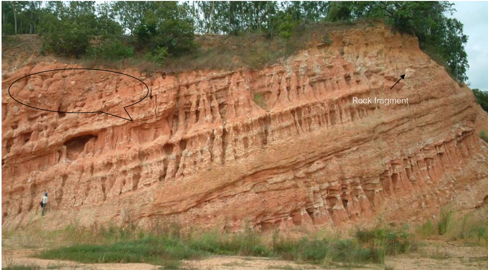
Figure 4.20 Alluvial fan sequence at the southern part of Khao Din (Sri Racha area) with bedding planes 196/15 W (Strike/Dip). Grid reference 0711932 E 1450139 N.
