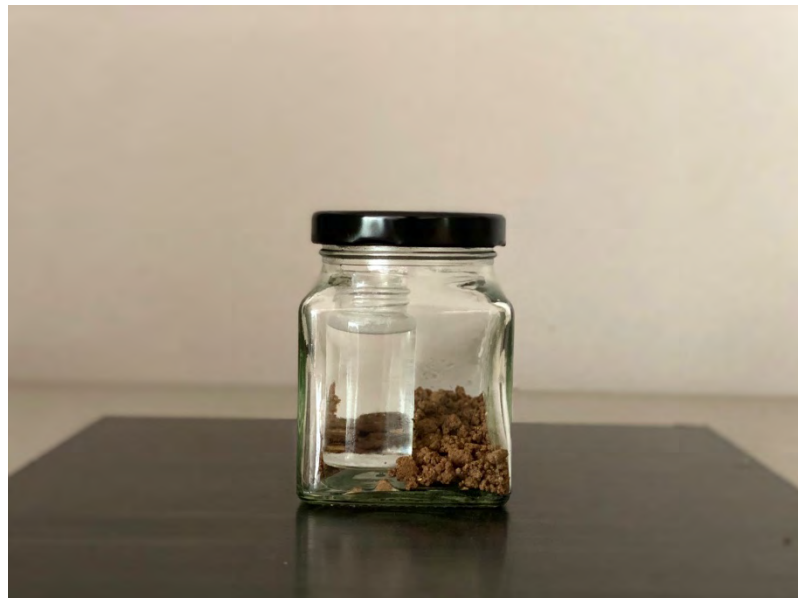
Figure 3.2 Biodegradation microcosm set-up
