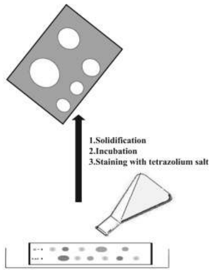
Figure 17: Diagram of immersion bioautography process
