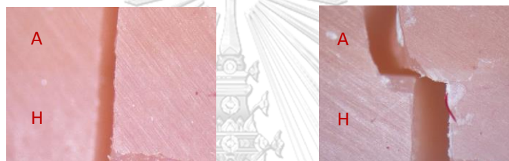
Figure 7. Specimens' fracture characteristic and chart presented number of each fracture characteristics (pcs). A: auto-polymerizing acrylic resin, H: heat-polymerizing acrylic resin.
