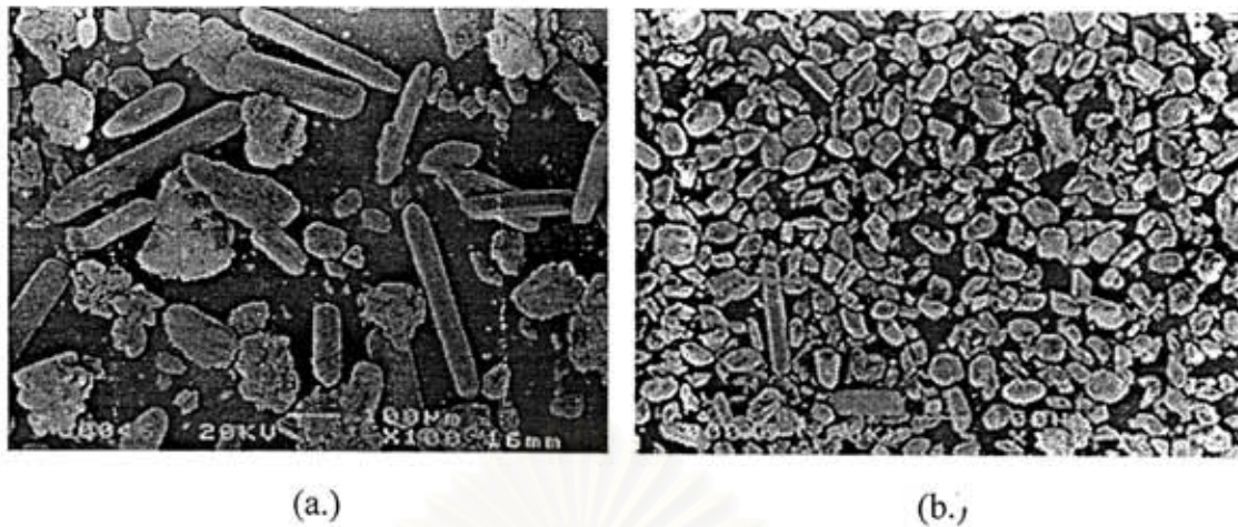
Fig. 3.3 SEM micrographs of a.) FGD (as-received) and b.) precleaned FGD
