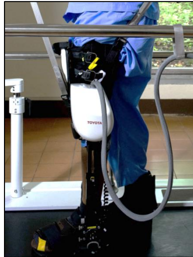
Figure 7 A knee-ankle-foot robot/robotic orthosis
