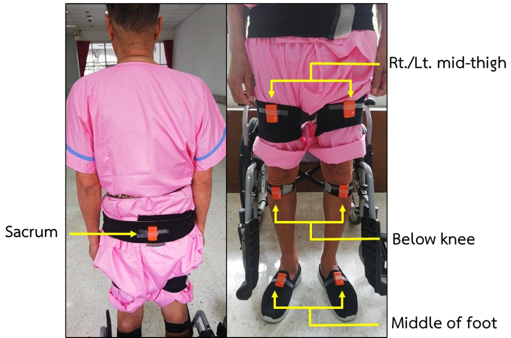
Figure 12 The placement of XSENS sensor
