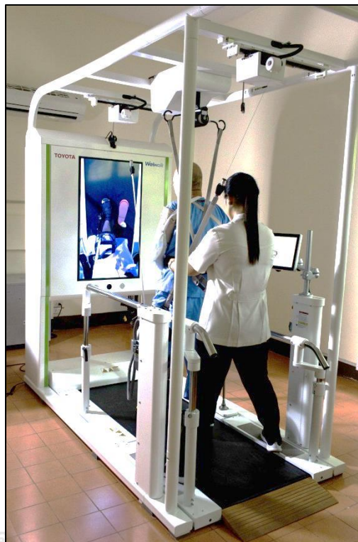
CHULONGKORN UNIVERSITY Figure 5 The Gait Exercise Assist Robot (Welwalk ® )
