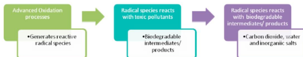
Figure 3 Schematic diagram explaining the processes involved in AOPS [11]
