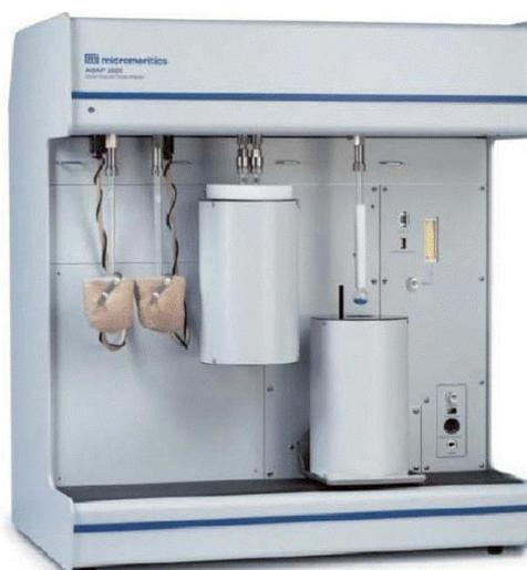
Figure 3.3 Micromeritics ASAP 2020.
