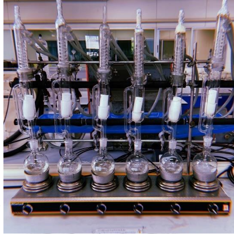
Figure 3.5 The chicken breast powder samples in the thimbles in a Soxhlet extractor
