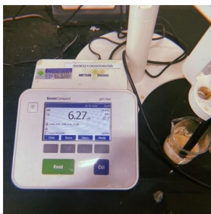
Figure 3.7 pH determination of chicken breast powder using seven compact pH meter
