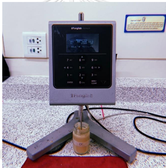
Figure 3.12 Pancake batter viscosity determination using Fungilab premium viscometer
