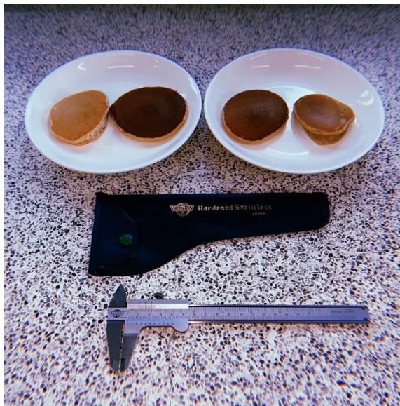
Figure 3.13 Determination of diameter and height of pancake samples using Kanon hardened stainless vernier caliper
