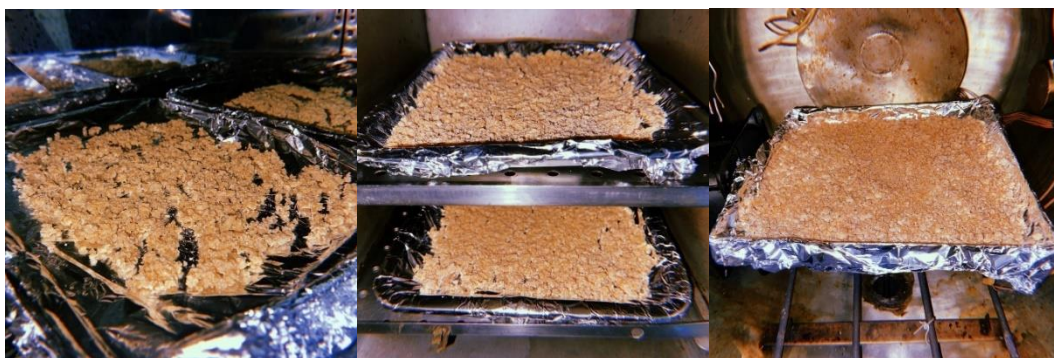
Figure 4.1 Dried chicken breast meat from different drying methods: conventional hot air drying (left), vacuum drying (middle), and low pressure superheated steam drying (right)
