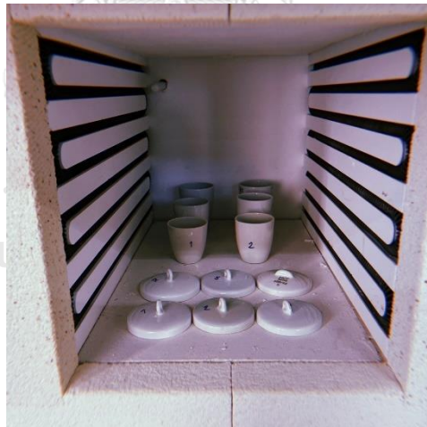
Figure 3.6 The chicken breast powder samples in the crucibles in a muffle furnace
