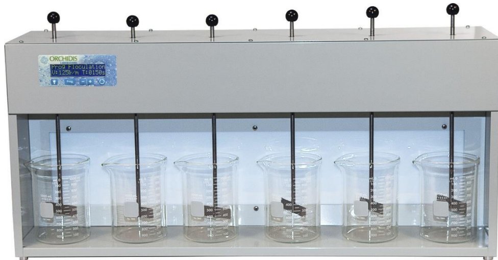
Figure 2.2. Jar test flocculator
