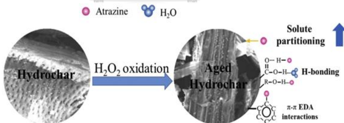
Figure 5. Mechanism of atrazine adsorption on aged hydrochar
