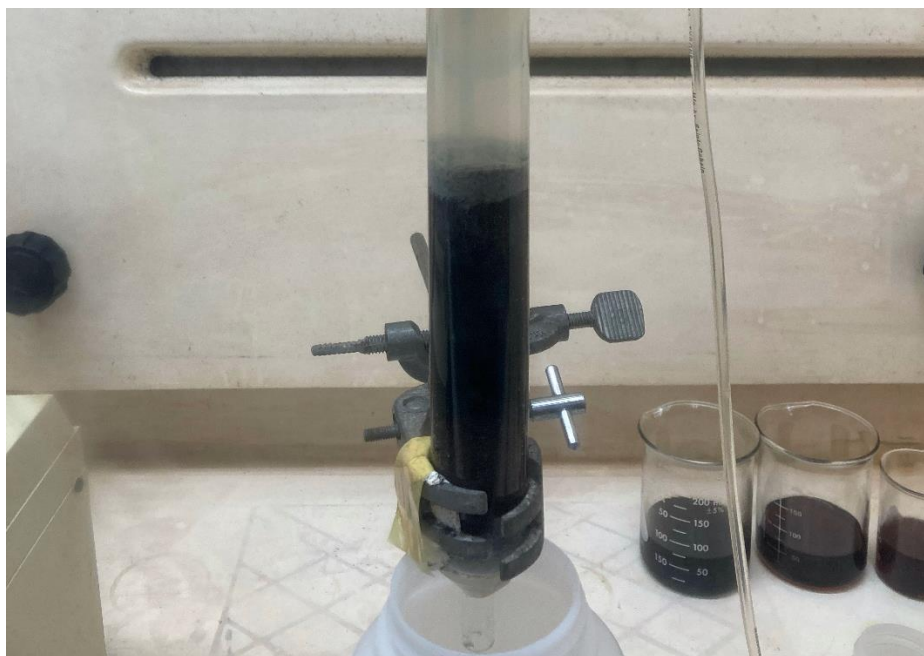
Figure B-5 Fixed bed column had clogged before reached breakthrough point
