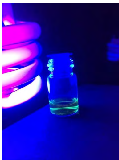
Figure 3.7 : Fluorescence of synthesized CdS QDs under UV light
