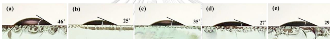
Figure 66. Contact angles of the PTAA films; (a) pristine, and post-treated PTAA by washing with 200 \mu\text{l} of DMF and followed by (b) 50 \mu\text{l} TO, (c) 75 \mu\text{l} TO, (d) 50 \mu\text{l} CB and (e) 75 \mu\text{l} CB.
