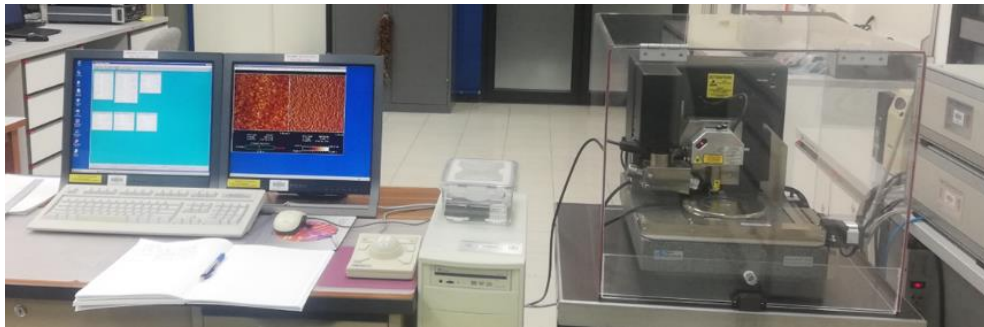
Figure 32. An atomic force microscope (AFM) on the right with controlling computer on the left.
