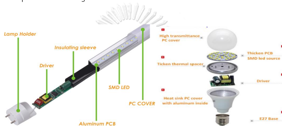
Figure 3.1 : Structure of selected LED models
