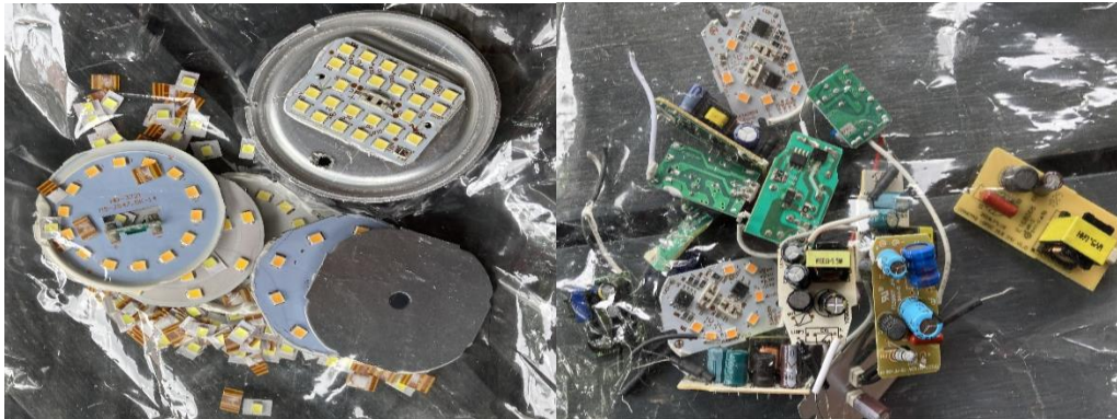
Figure 3.2 : LED drivers and sources from selected models.
