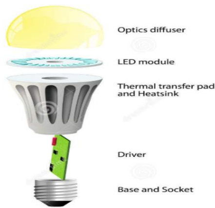
Figure 2.1 : Basic components of LED bulb (Philips, 2019)
