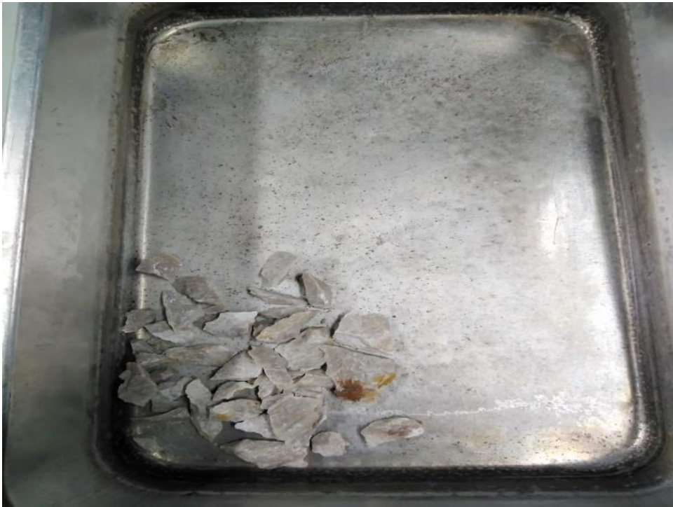
Figure 3.12 Crushed samples for XRD and XRF
