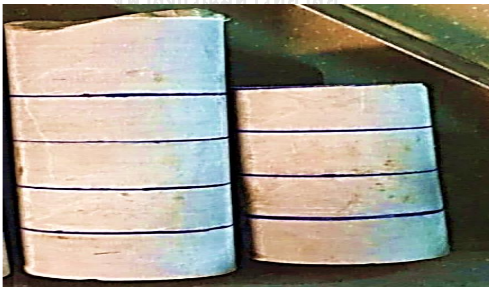
Figure 3.8 Prepared core samples for UCS
