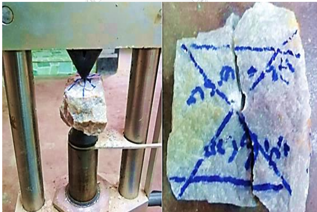
Figure 3.6 Sample after point load test
