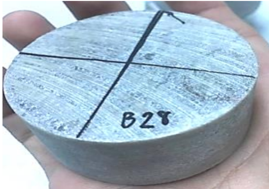
Figure 3.10 Prepared samples for Brazilian test
