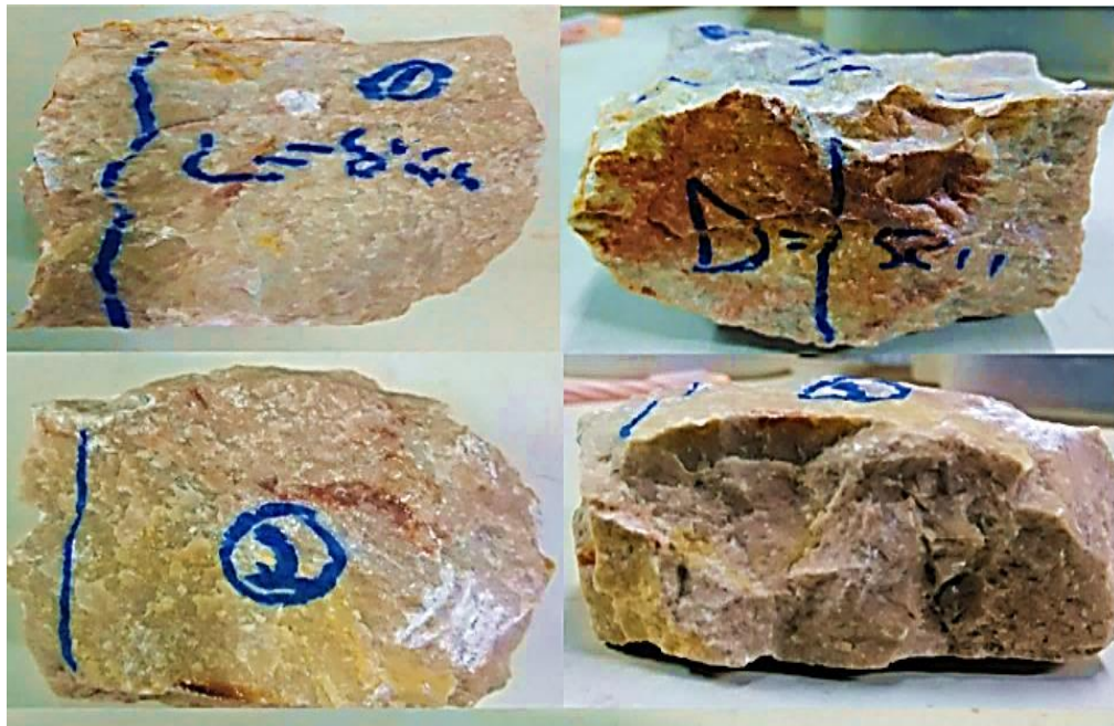
Figure 3.5 Prepared samples before point load test
