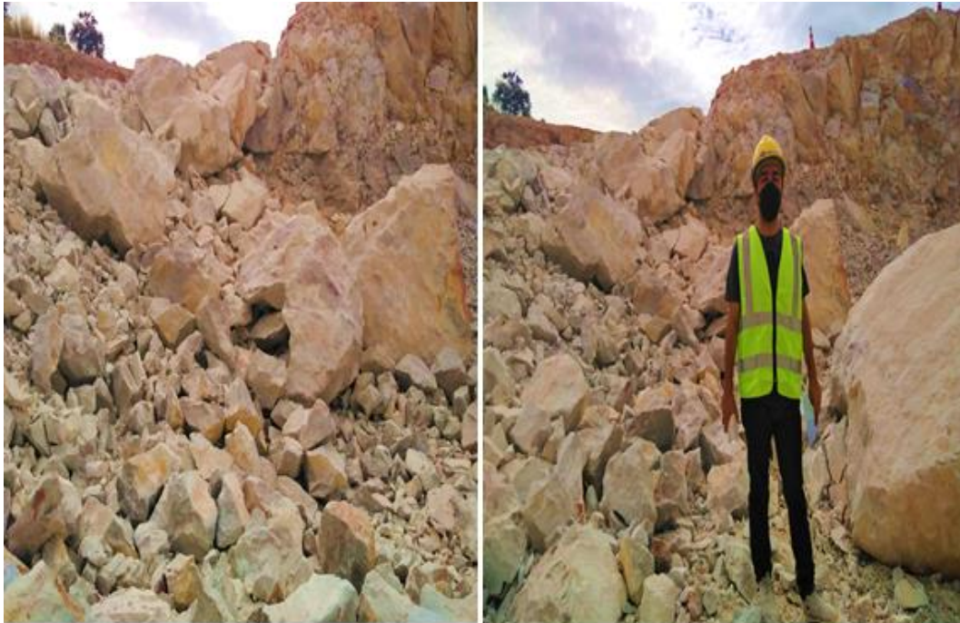
Figure 1.1 Unwanted boulders after blasting at Pyrophyllite quarry
