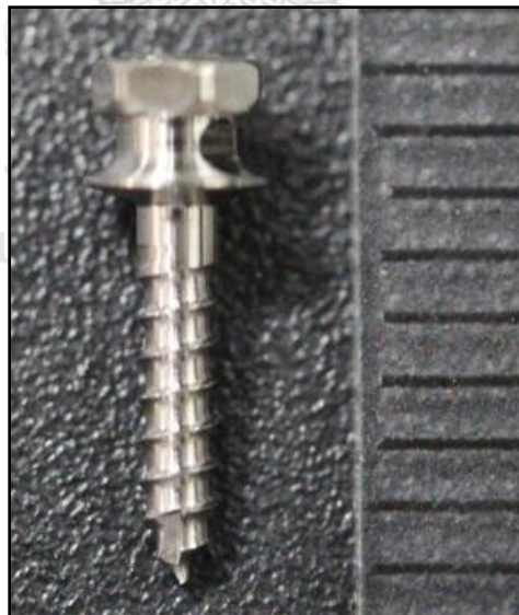
Figure 14 An image of Ti6Al4V miniscrew used in this experiment (1 scale = 1 mm).
