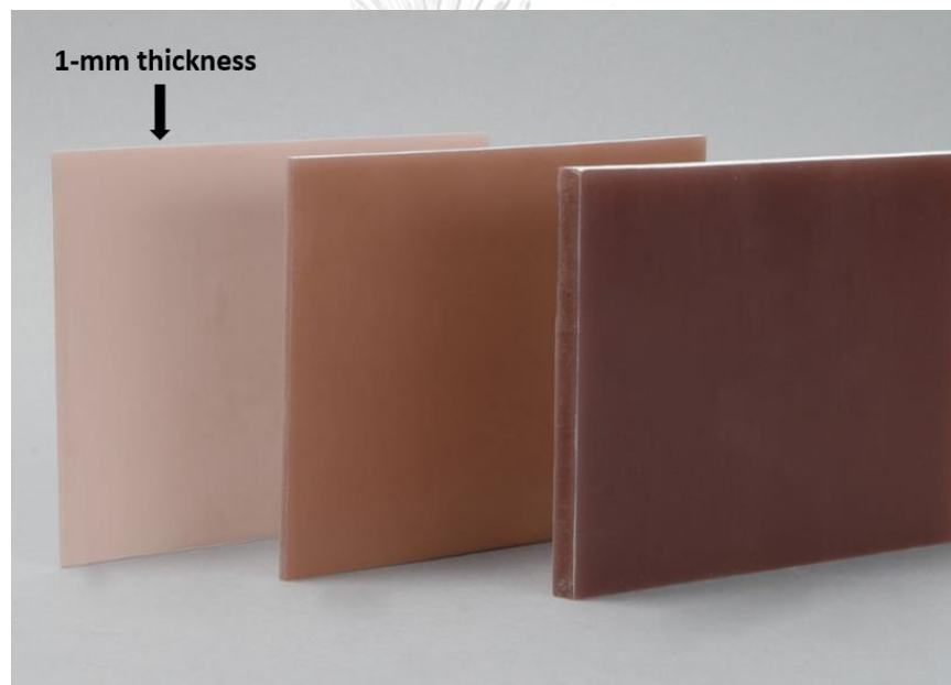
Figure 13 a 1-mm thick E-glass filled epoxy sheet (pale pink) used in this experiment
