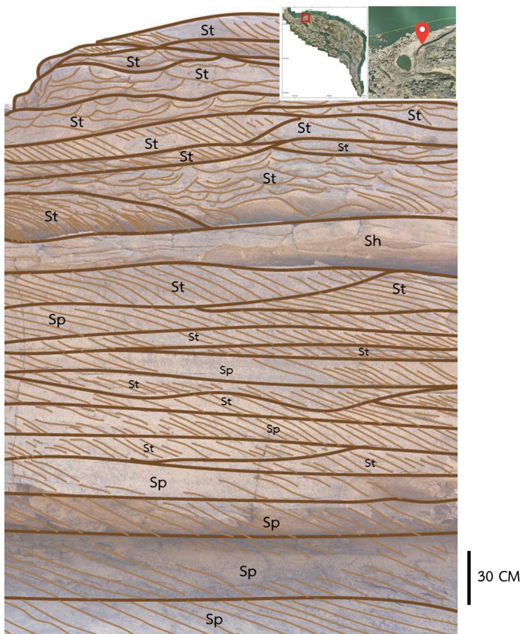
Figure 5.11 The photo shows the lithofacies in the Phu Phan formation sandstone at the Samphanbok. Sp facies show sandstone with planar crossbedding and St facies show sandstone with trough crossbedding.
