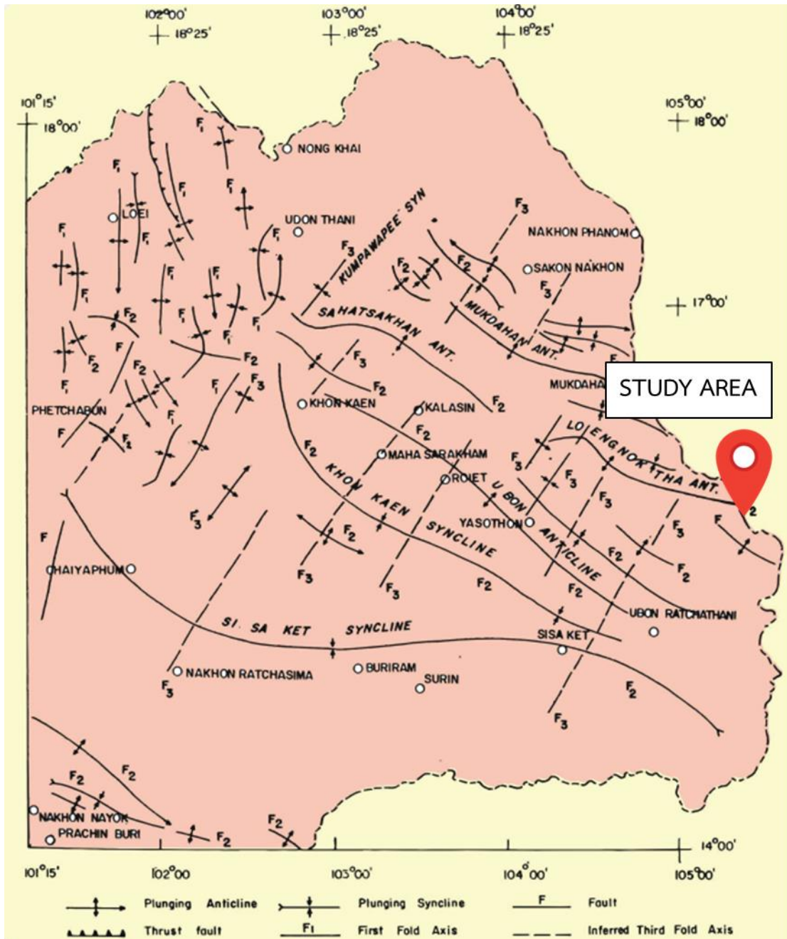
Figure 1.5 The map depicts the structural geology of Mesozoic rocks resulting from tectonic events in the Indochina plate. (Chuaviroj, 1997)
