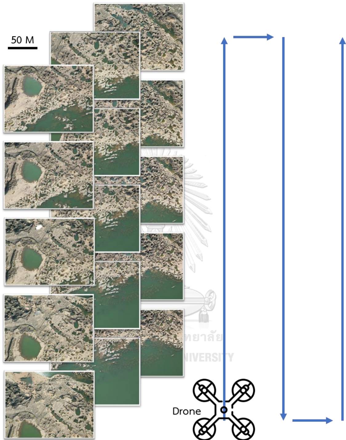
Figure 3.7 The image displays the grid pattern pathway followed by the drone to capture photos with a minimum of 60% overlap.
