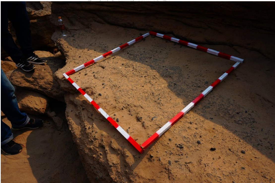
Figure 3.10 The photograph depicts the process of counting pebbles in a horizontal plane within the sandstone bed.
