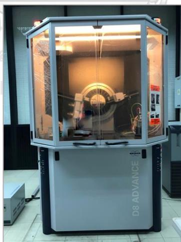
Figure 3.19 X-ray diffraction spectrometer
