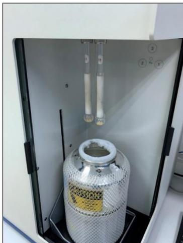
Figure 3.16 N<sub>2</sub> physisorption measurement
