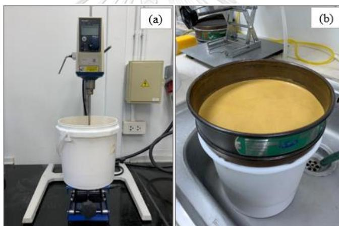
Figure 3.12 Purification setup process; (a) Mixing, (b) Sieve
