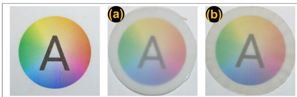
Figure 39. Cellulose films obtained from fibers treated with ZnCl 2 -LA at 110 °C for: (a) 30 minutes and (b) 120 minutes
