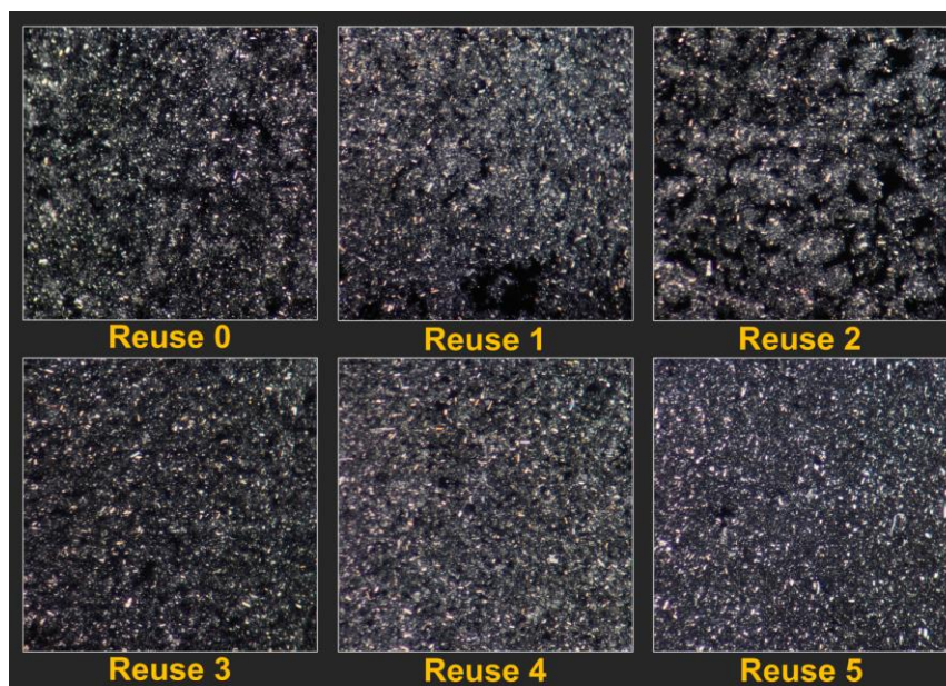
Figure 41. PLM images of CMNF fibers obtained by SCB pretreated with reuse DES.
