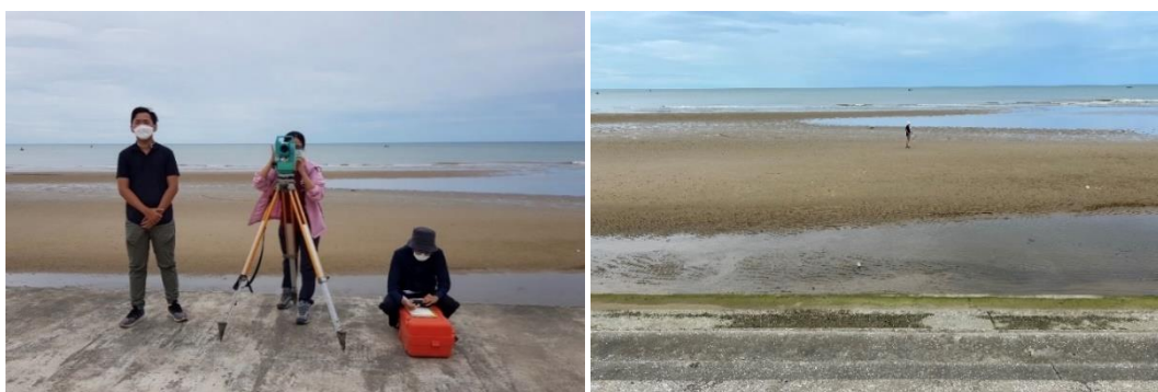
Figure 16. Coastal measurement conducts by Total Station camera.
