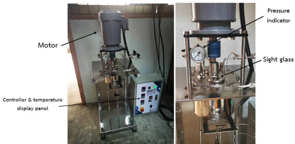
Figure 4.5 Picture of the designed and fabricated centrifugal
