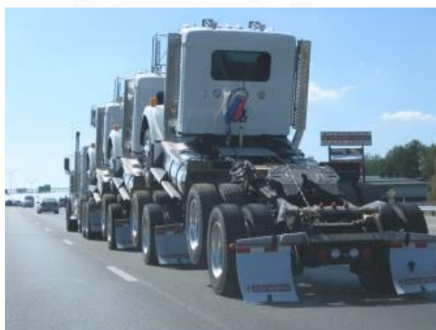
รูปที่ 12 Saddle-Mount Truck Tractor Unit Operating along IH 35 SB—Austin District
