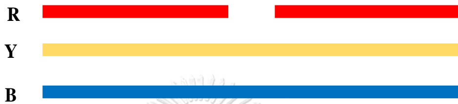
Figure 6 Single-phase open fault
