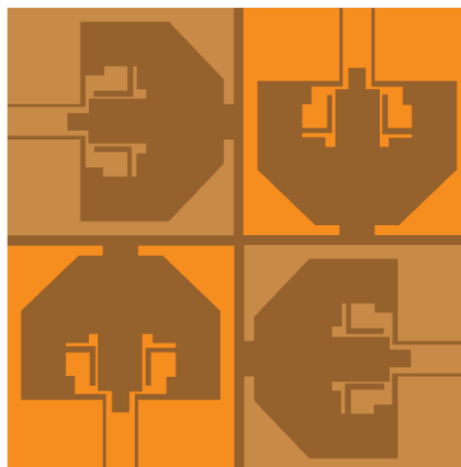
Figure 31: Complete structure of antenna with four antenna elements on either side of the substrate.
