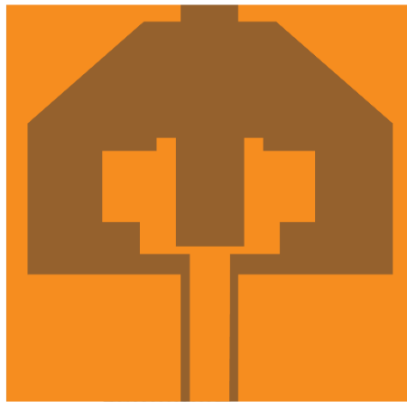
Figure 28: Individual Antenna element with radiator and ground.
