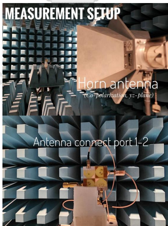
Figure 46: Fabricated Model of the proposed MIMO antenna being tested in Anechoic Chamber in YZ-plane.
