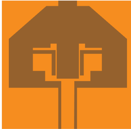
Figure 29: Individual Antenna element with inverted L shaped notching elements on the radiator.
