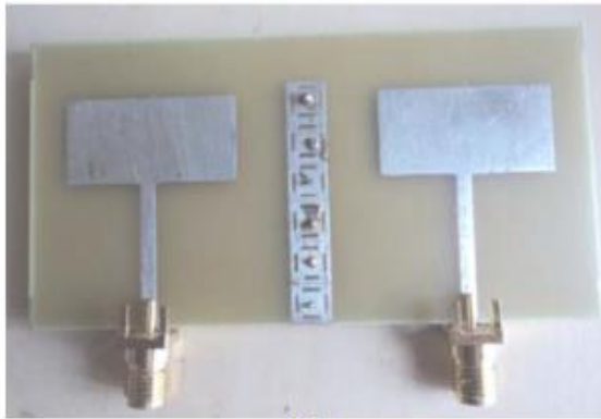
Figure 17: Parasitic elements used between antenna radiators.
