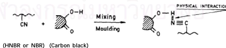
**Figure 4.5** Probable mechanism of bonding in HNBR or NBR with carbon black system [22].
