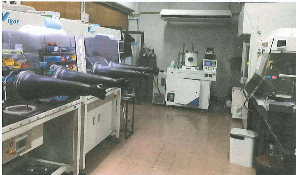
Figure 4 Left (glovebox) where the perovskite layer is formed (middle) thermal evaporator (right) fume hood with a spin coater for ETL/HTL layer formation.
