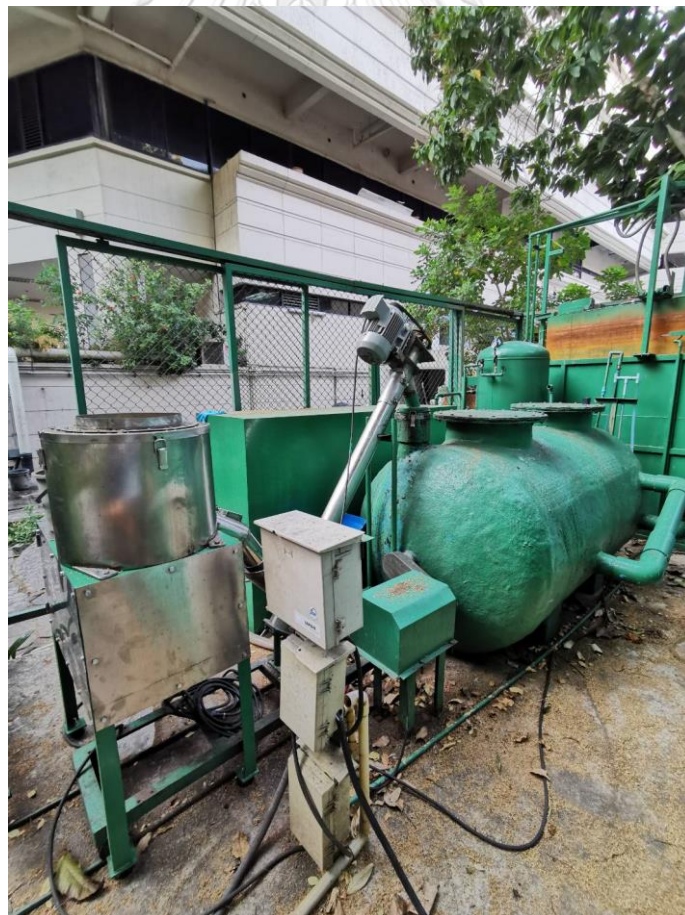
Figure 8 Shredder and screw conveyor
