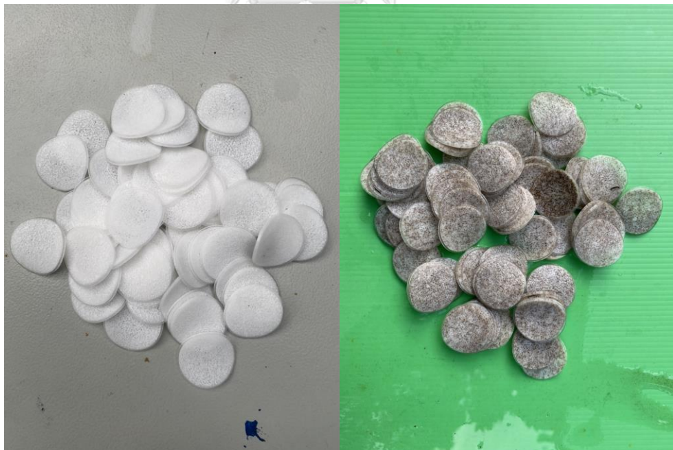
Figure 25 Biofilm carrier (MBBR media) comparing the new MBBR media and the active MBBR media
