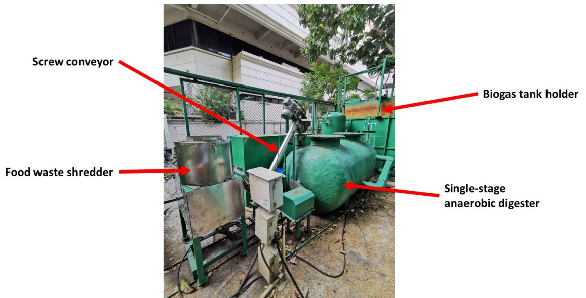
Figure 15 Overview of the food waste treatment system using in the zero-waste
