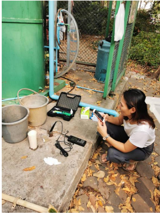
Figure 28 Onsite measurement of wastewater samples
