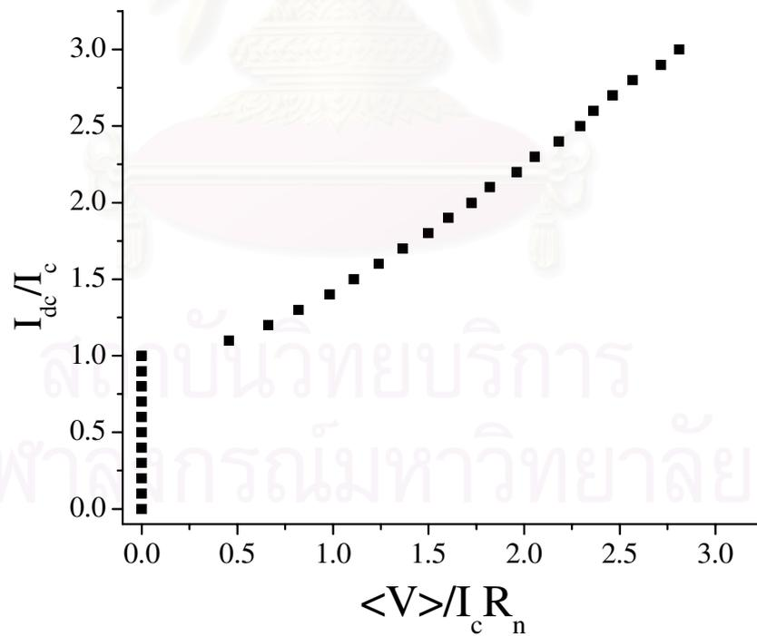
Figure 3.8: The current-voltage characteristic of Josephson junction with  $\beta = 0.1$ .
