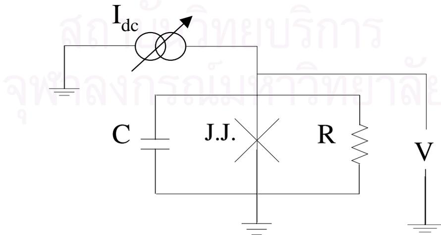
Figure 3.2: The equivalent circuit diagram of Josephson junction.
