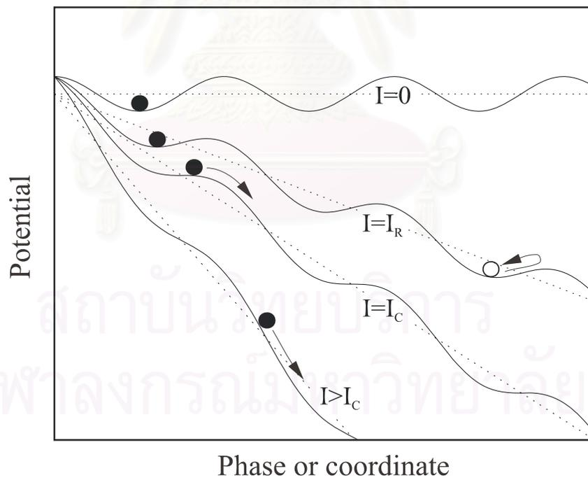
Figure 3.12: Model of a massive particle moving in the tilted washboard potential[14].
