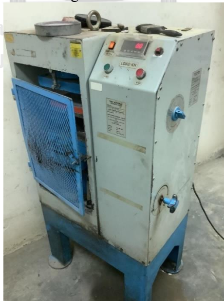
Figure 19 Compressive strength machine
