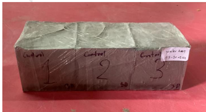
Figure 18 Curing cement samples
