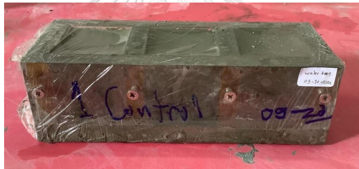
Figure 17 cement paste in mold cover with plastic sheet
