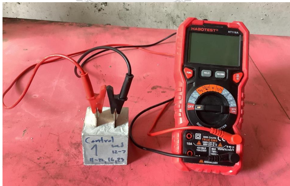
Figure 20 Electrical conductivity measurement using digital multimeter.
