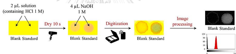
Figure 2.7 Schematic representation of the experiment procedure for boron detection [18].
