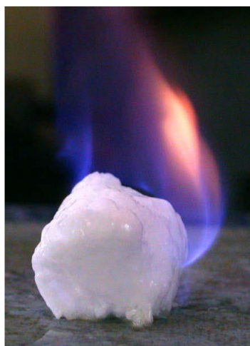
Figure 2.1 Burning of methane hydrate sample (Siažik et al. , 2017).
