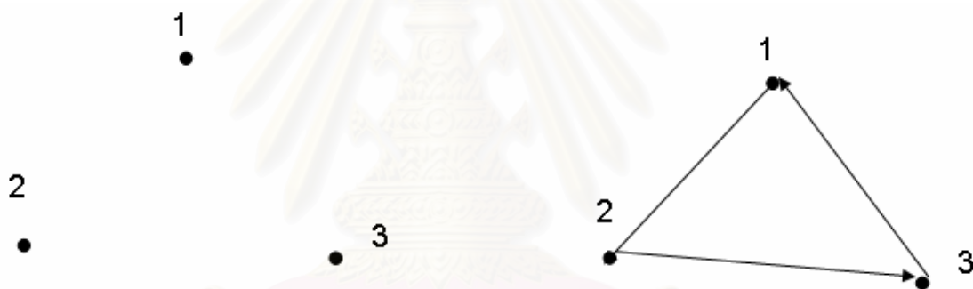
Figure 2-4: Primitive assembly steps. From this Figure, each vertex is connected together in a specific order to form a geometric primitive.
