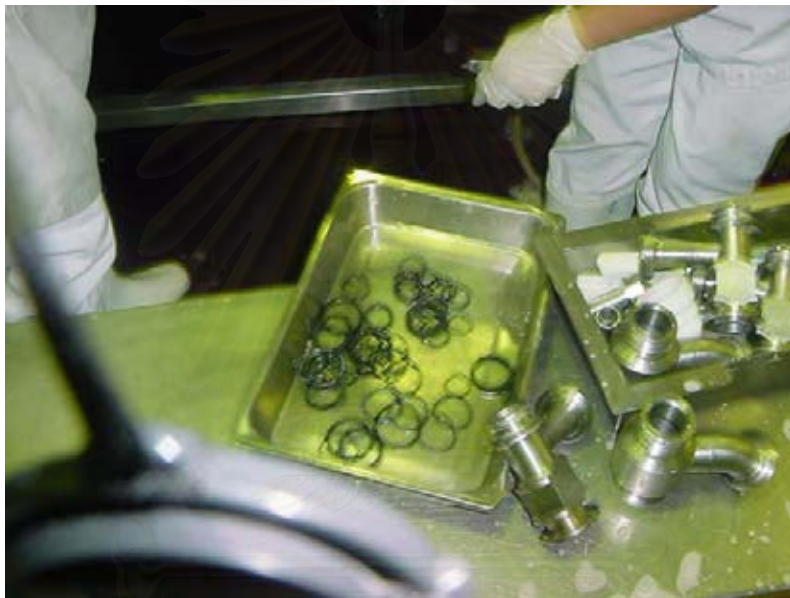
Figure 4.35: Existing o-ring's cleaning process
