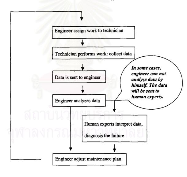
Figure 1.1 Process of vibration signal in maintenance work.
