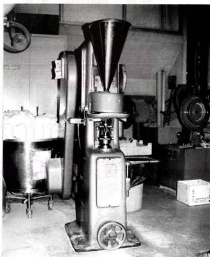
Figure 5.3 Heavy duty single stroke tableting machine
