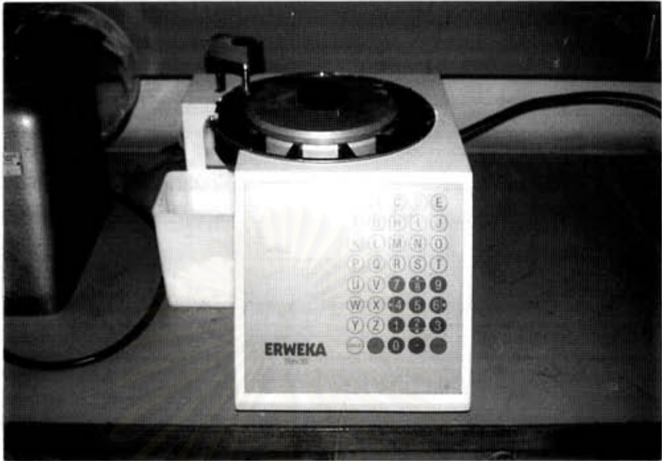
Figure 5.6 Erweka TBH 30 (for measuring hardness and diameter of tablet)
