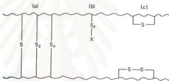
Figure 2.3 Structural features of vulcanisate network [14]
